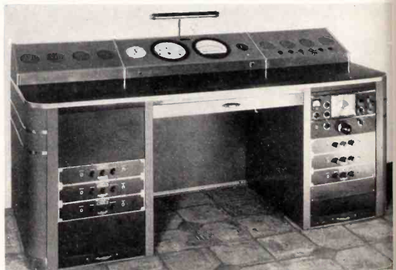
New radio traffic control console designed for Miami's 36th Street airport. Features include roll-out receiver racks facilitating maintenance
