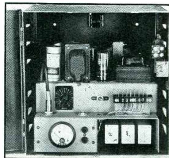
Fig. 7—Holmes a-c amplifier, band-pass filter and power supply unit. (Photo-tube detector "head", not illustrated, is mounted few feet away.) Plug at lower left may be removed and inserted in jack few inches to right to test performance of system without a-f filter. One of three relays visible at lower right may be tripped from remote office to extinguish lightsource and check system performance
