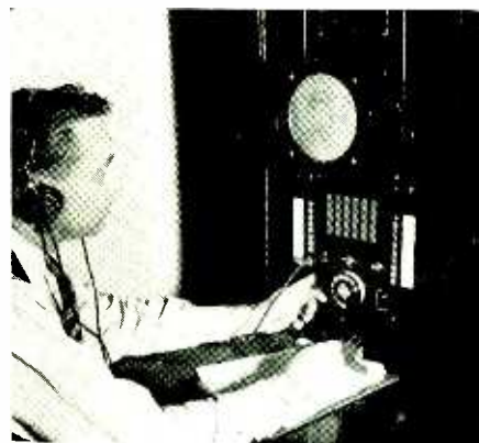
The azimuth indicator in use at LaGuardia Airport. The indication appears on the cathode-ray tube screen
