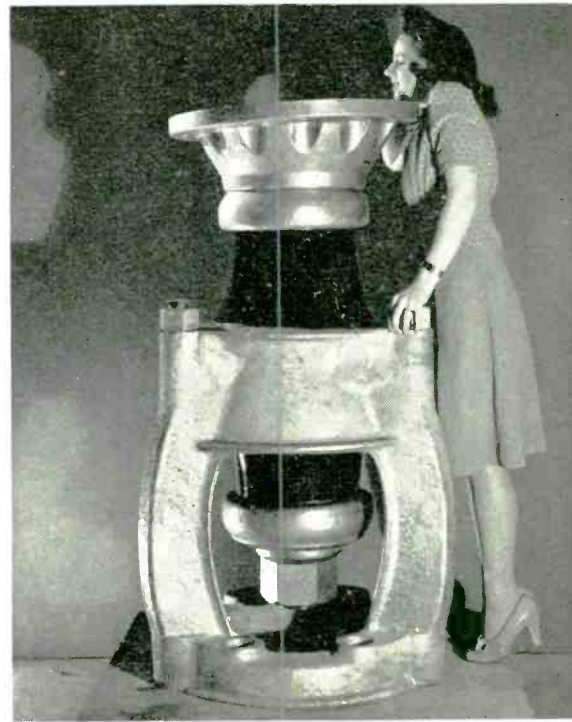
One of the WABC tower footing insulators before shipment from the Lapp factory. These curved-side compression cones of high-voltage porcelain offer remarkable electrical and mechanical characteristics. This insulator was tested at 780,000 pounds in the Lapp laboratory. No Lapp footing insulator has ever failed in service.
