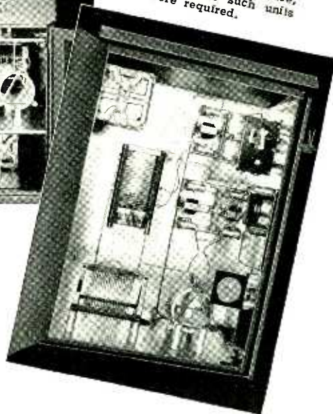
Antenna Coupling Unit for WTMJ, Milwaukee Journal, Milwaukee, Wis. Three such units were required.
