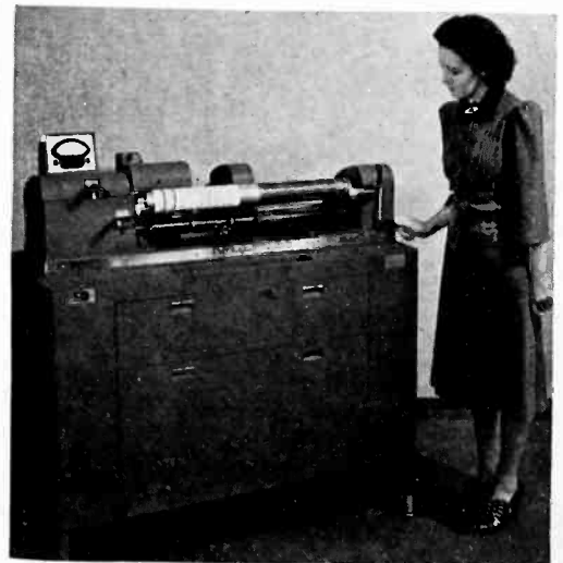
Multifax unit of Western Union, with which stencils, master plates and tracings are prepared from original copy
