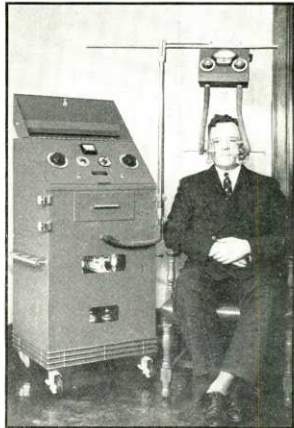
Apparatus for measuring diathermy dosage rate described by Kraus and Teed
