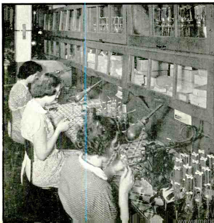
The larger tubes are tested at frequencies up to 100 megacycles in these oscillator units. If the quality of the tube is not up to standard, or if it is to be subjected to rough handling, an X-ray picture is made to check the alignment of the parts
