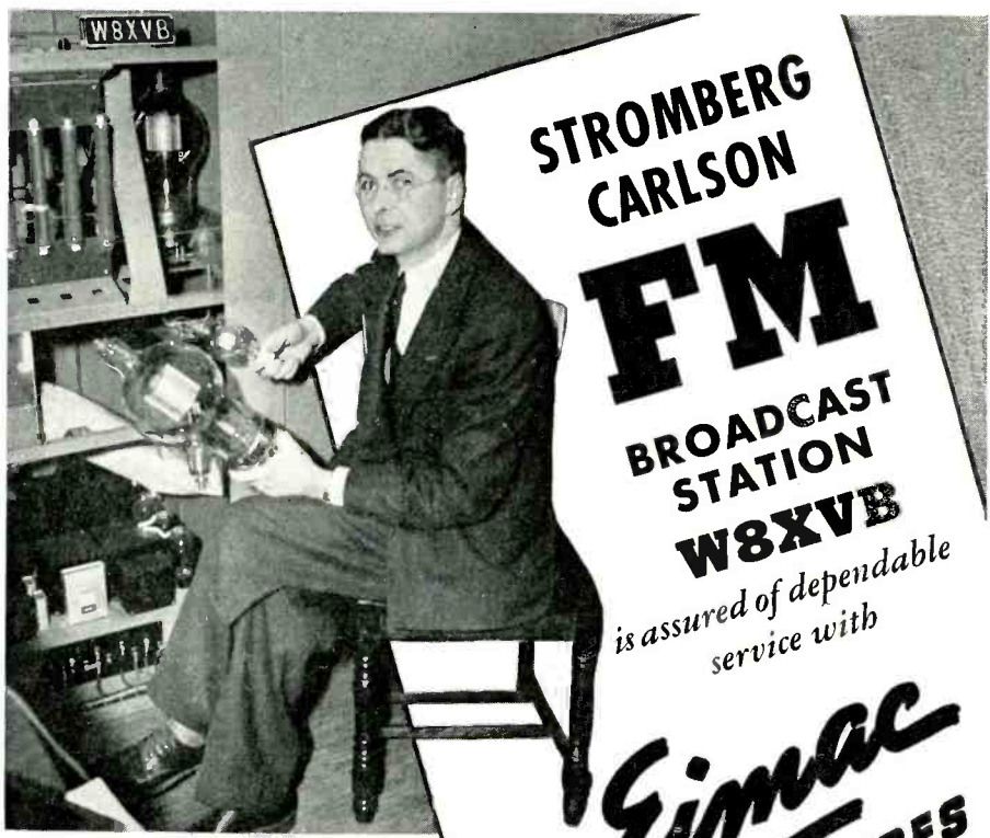
Technical supervisor of radio station WHAM and W8XVB, is seen holding one of the Eimac 1500T Tubes used in FM station W8XVB
