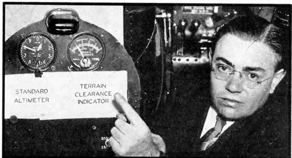
The two dials show the altitude indications of a barometer-type meter (left) and u-h-f reflection-type indicator. With only 100 feet actual clearance, the barometer shows 800 feet altitude above sea level
