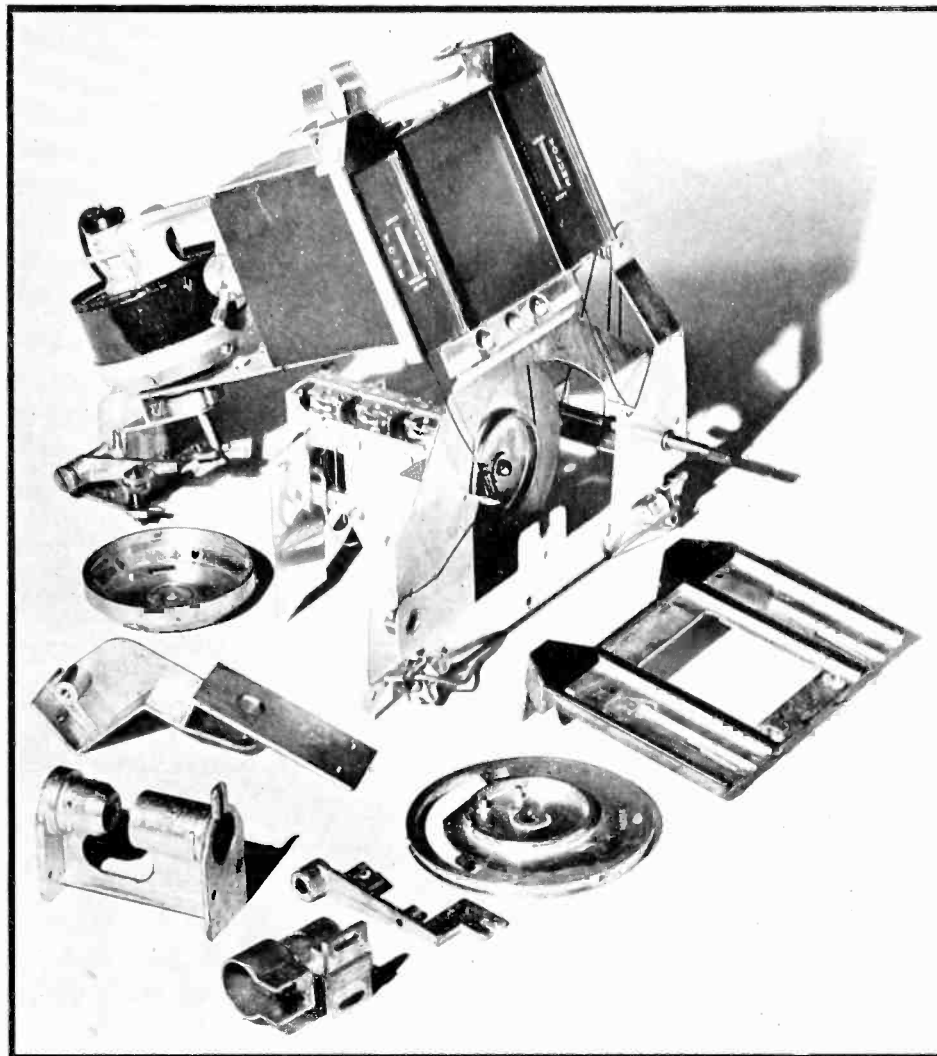
The "Movie Dial" is the dark colored cylinder of film in left background, an image of portions of which is projected on ground glass in top center panel. Die castings used in the assembly of the unit are shown separately in the foreground
