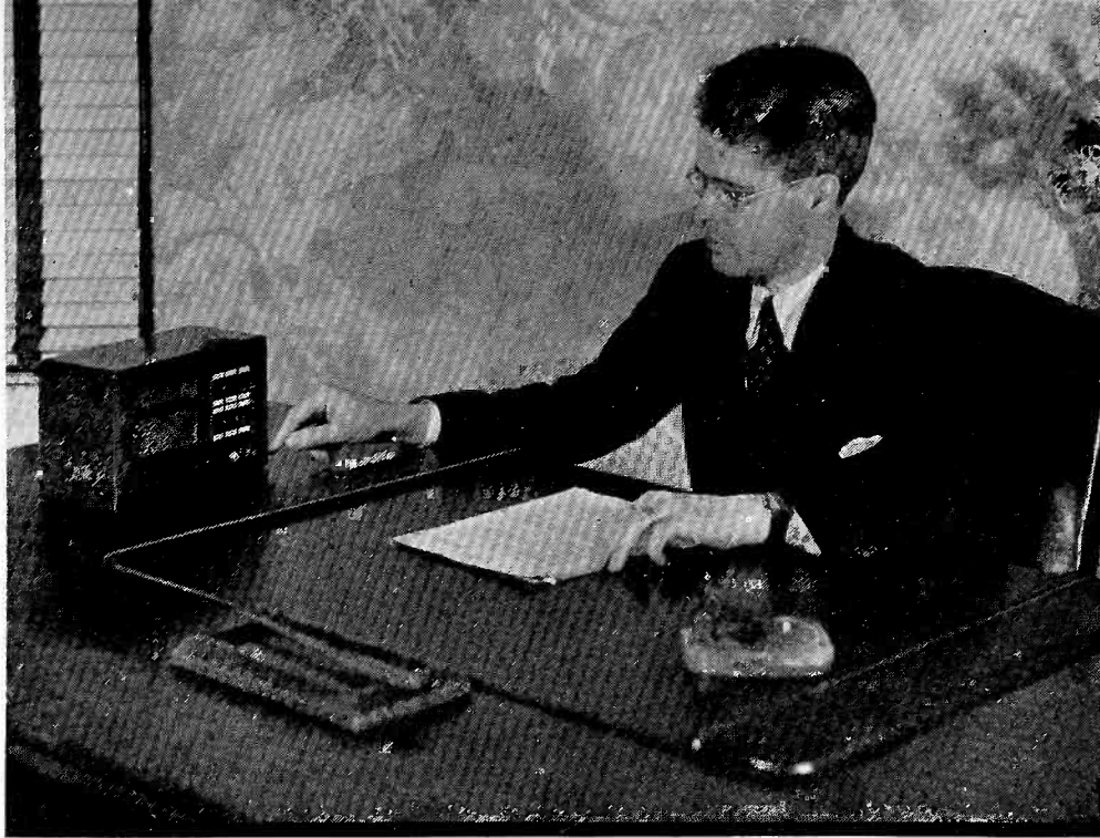
The master station can be connected with any outlying station, each of which can talk back when the master is switched to "listen"
