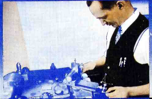
Sawing the crystal blanks at the proper angle is the first important step.
