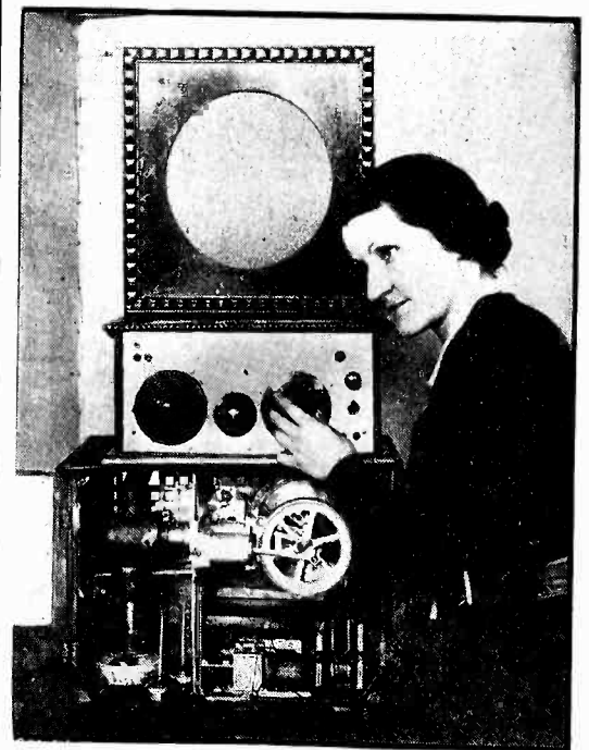
The batteries of this German radio set are charged by a small hot-air motor-generator, which derives its power from a kerosene lamp (lower left)
