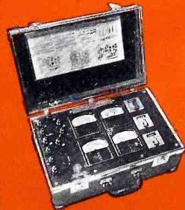
INDUSTRIAL ANALYZER—Self-contained for making complete a-c. tests up to 125 amperes, 600 volts on single, two, or three-phase circuits.
