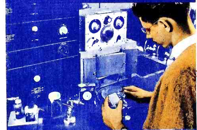
Measuring the finished blanks on micrometer for final check-up on frequency.
