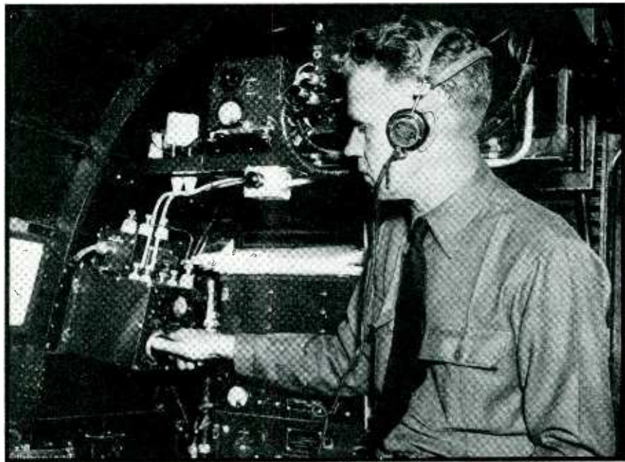
Two radio transmitters, using phone, CW, and ICW, are installed in the new 205-mile-an-hour Douglas twin-motor plane which serves as a flying headquarters for Major General Frank N. Andrews, commander of the GHQ Air Force. One set has a range deliberately limited to 25 miles for liaison communication with nearby squadrons on fighting ships, the other has a normal reliable range of 750 miles. A "homing" compass radio direction finder and a robot pilot are included in the equipment of the plane
