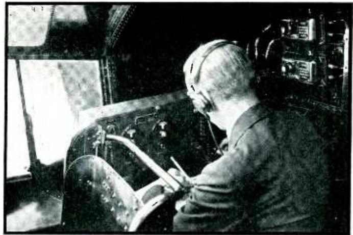
Two views of the equipment in a Sikorsky plane. The receiver, key, power switches and battery chargers are directly under the operator's control. The transmitter is remotely controlled
