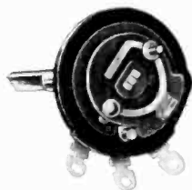
Internal construction of the Midget Control showing design of contact carrying mechanism.
