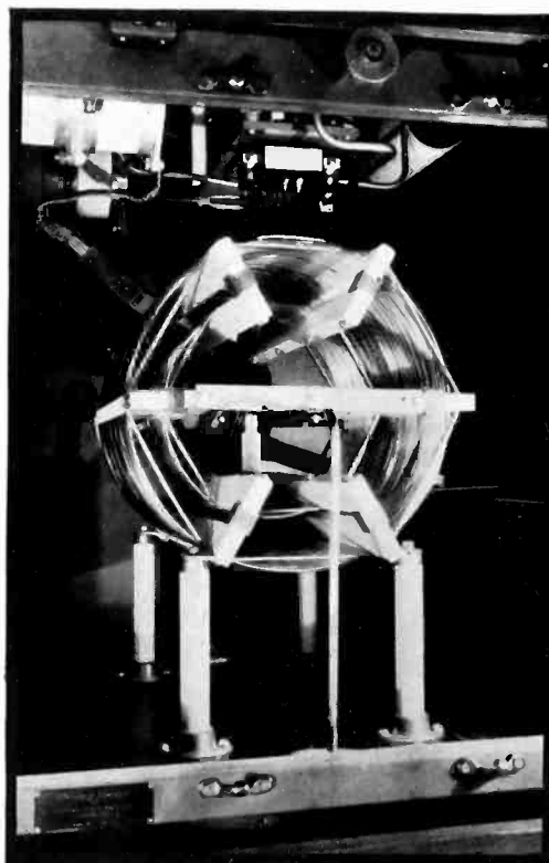
Power amplifier and output circuit—tuning control (at top) operated by key prevents inadvertent detuning
