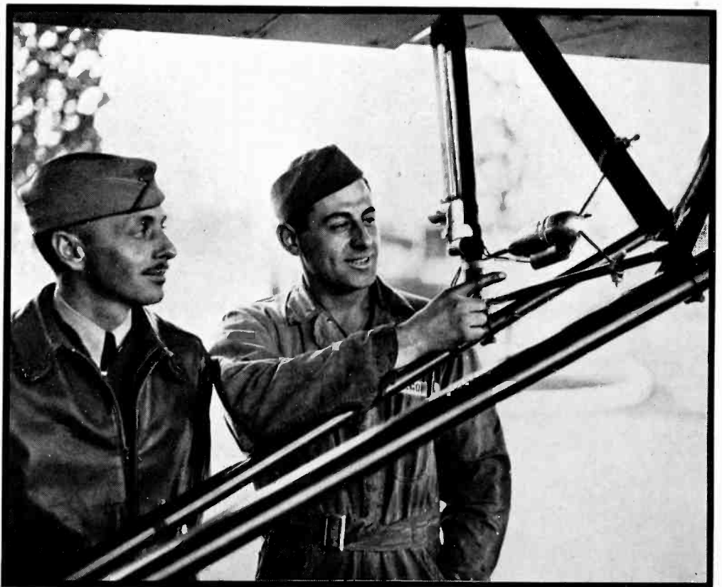
A radio meteorograph of the Blue Hill Observatory, Harvard University, is carried aloft 17,000 feet each day by Pilot A. V. Marsh and his assistant R. De Gregorio. The instrument radios the barometric pressure, temperature and humidity automatically to the observatory below
