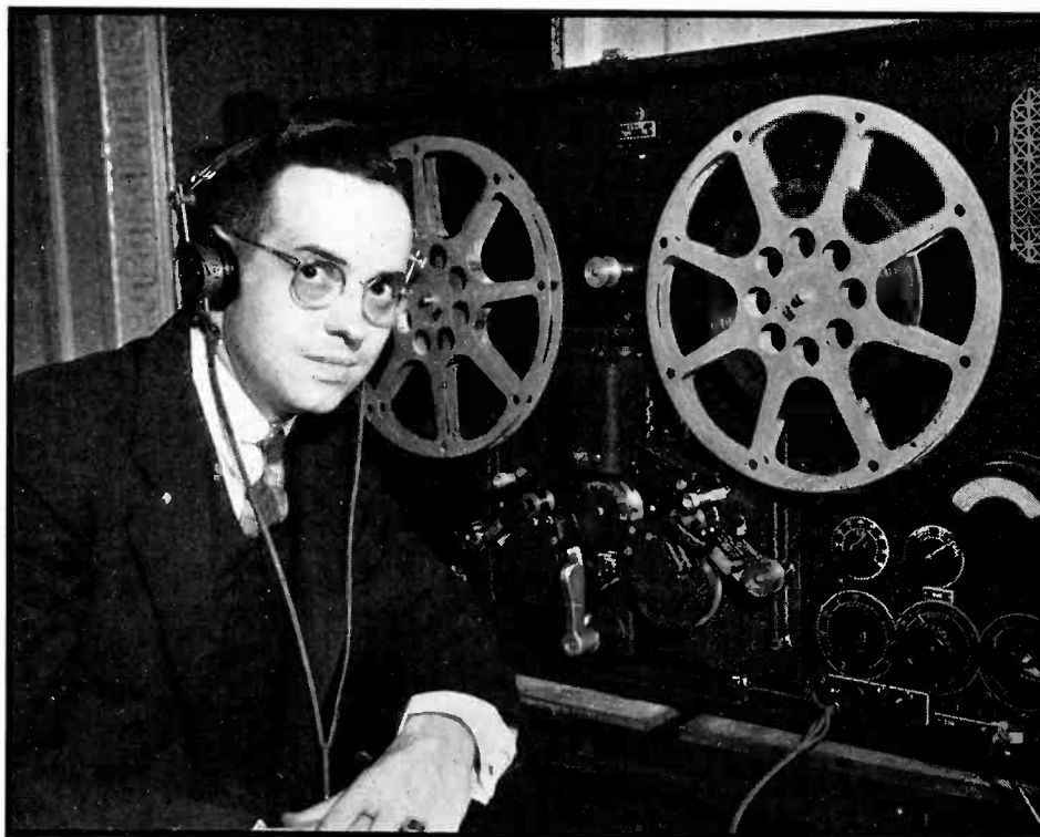
A new device for recording conversation and other evidence secretly by means of a diamond stylus engraving on celluloid film. The recording may be played back immediately without processing
