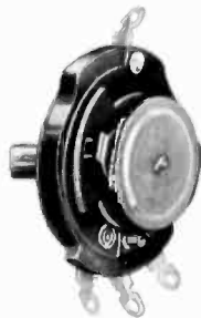
Type "P" Control with metal cover removed showing addition of friction clutch to standard tap type control.
