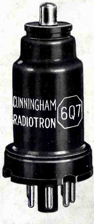
DUPLEX-DIODE HIGH-MU TRIODE —Heater Current 0.3 ampere. Triode Amplification Factor 70.
