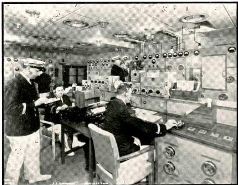
The communication center of this great ship contains every possible facility for marine radio, even to complete soundproofing of the room
