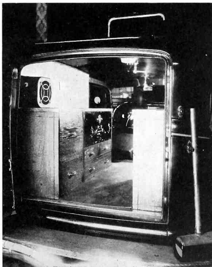
Interior of radio-interference car, showing control panels, battery cabinets, loudspeaker, etc. The heavy mallet at right is used to jar pole-line structures, and thus show up interference sources
