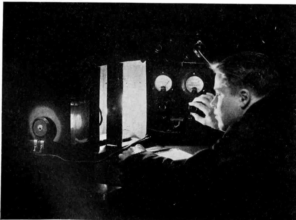
With the aid of this Westinghouse photoelectric apparatus for measuring transparency, G. W. Holmes studies sewage turbidity for the city of Syracuse, N. Y. The method can also be applied for sewage treatment operations involving automatic control
