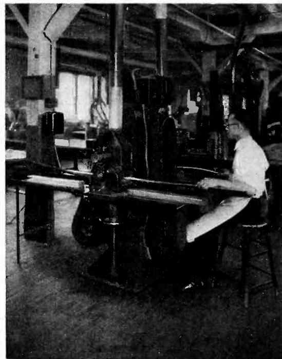
A G-E photoelectric relay was put to work counting sheets of mica passing through this machine, and registering an exact count before the eyes of the operator. The saving in time and material more than justified the cost of the installation
