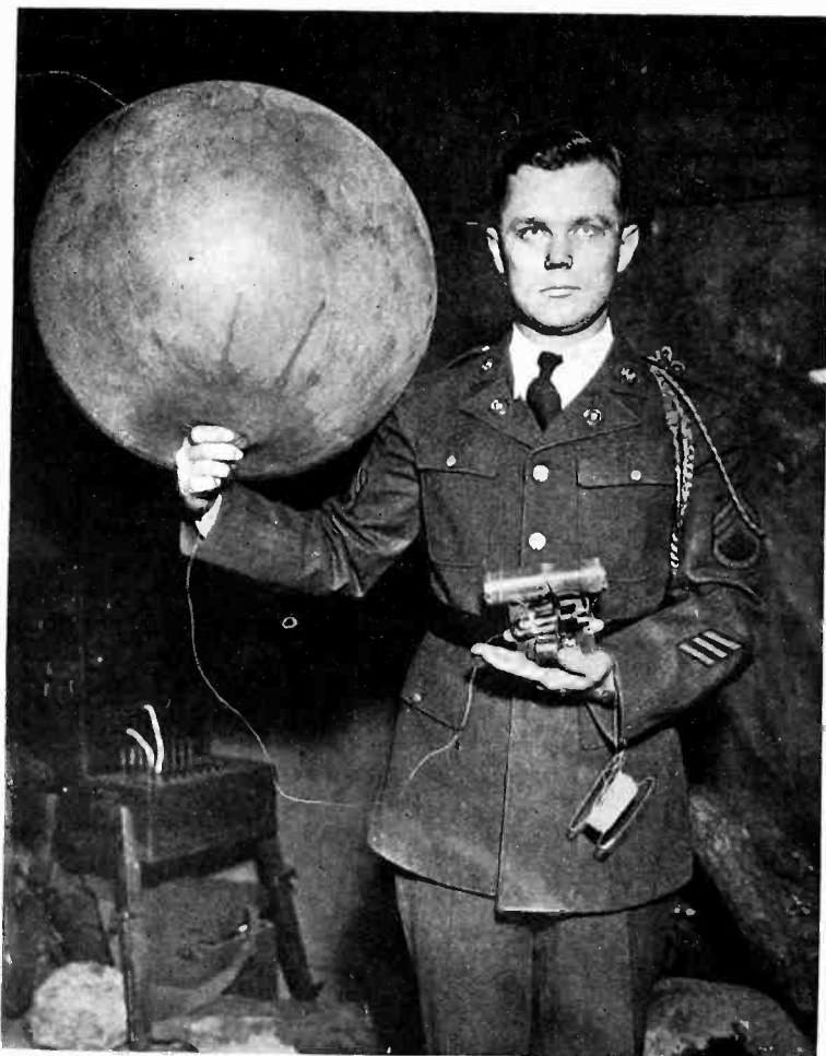
Compact one-pound transmitter built by Sergeant Milton A. Sewell of the Signal Corps for sending dots and dashes from meteorological balloon to give air conditions aloft
