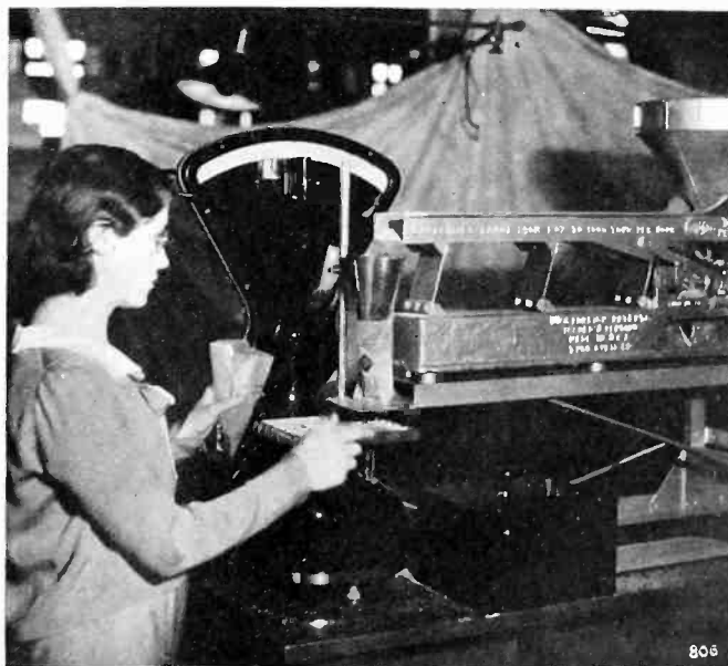
When the pointer on this Toledo scale reads proper quantity, the photo-cell cuts off supply of powder
