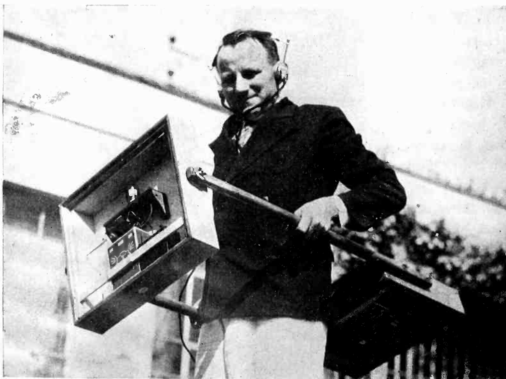
Presence of metal bodies within a depth of 10 feet and a radius of 5 feet is made audible by this device perfected by Gerhard Fisher. It weighs 22 lbs.
