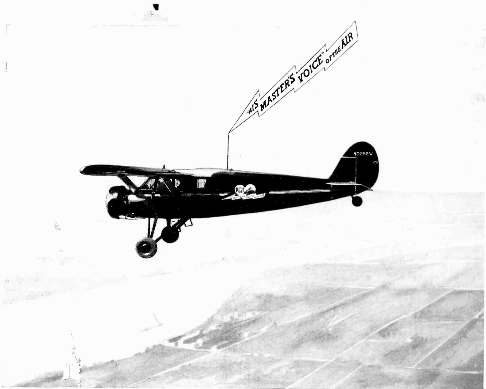
RADIO COMMUNICATION ON THE WING—The Stinson Junior cabin airplane used for testing and demonstrating RCA Victor aircraft equipment.
