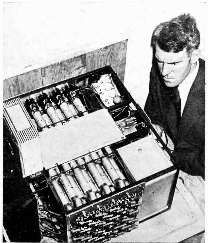
In this "hodoscope" built by Dr. Charles Johnson of Swarthmore, Pa.; the grouped Geiger counters operate corresponding neon lamps so that the angular direction of each high-speed cosmic-ray particle is clearly shown to World's Fair visitors
