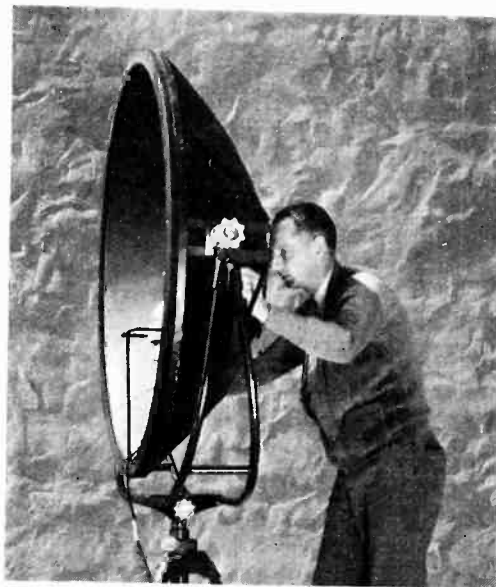
After revolutionizing Hollywood's talkies, the parabolic-reflector microphone picks-up opera, is tested out against senatorial oratory
