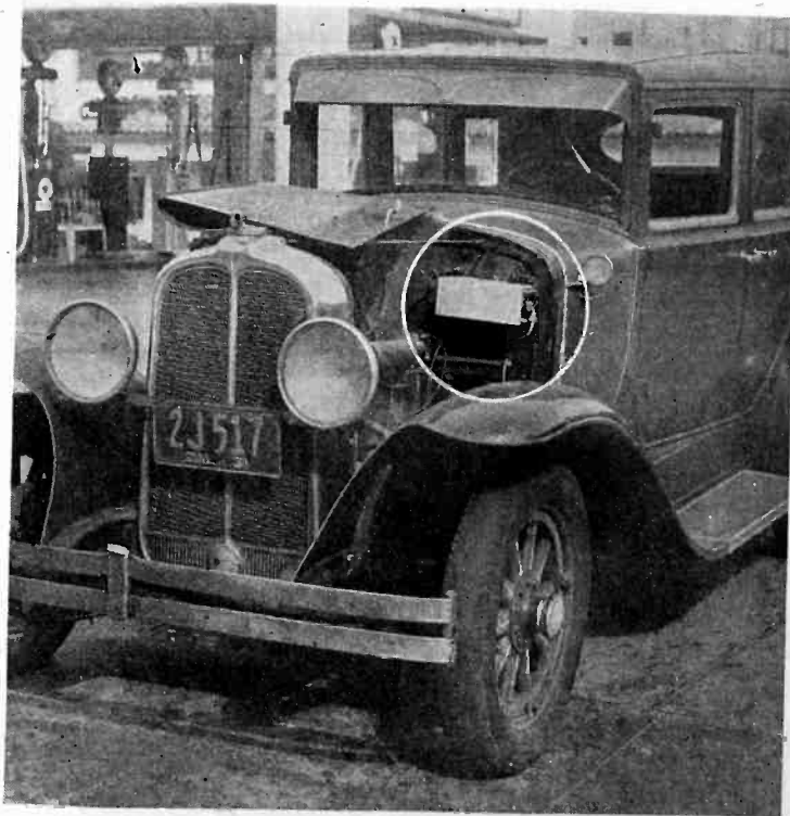
The Dynatope, Hutch-Gard, San Francisco, installed in a Pontiac Six. This is a non-rotating type of converter changing six volts d.c. to a.c. 110 volts
