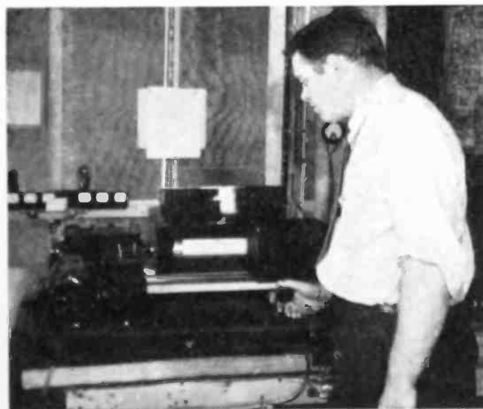
Apparatus for sending and receiving a small four-page newspaper to ships at sea using short waves, is now in regular use on the "Leviathan" and other American vessels. Receiving machines translate radio impulses to printers' ink on miniature pages
