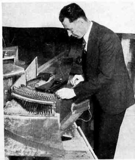
Drs. DuMond and Kirkpatrick of the California Institute of Technology designed this crystal spectrograph to show electrons in atoms of solid matter are in constant motion and move at high speeds
