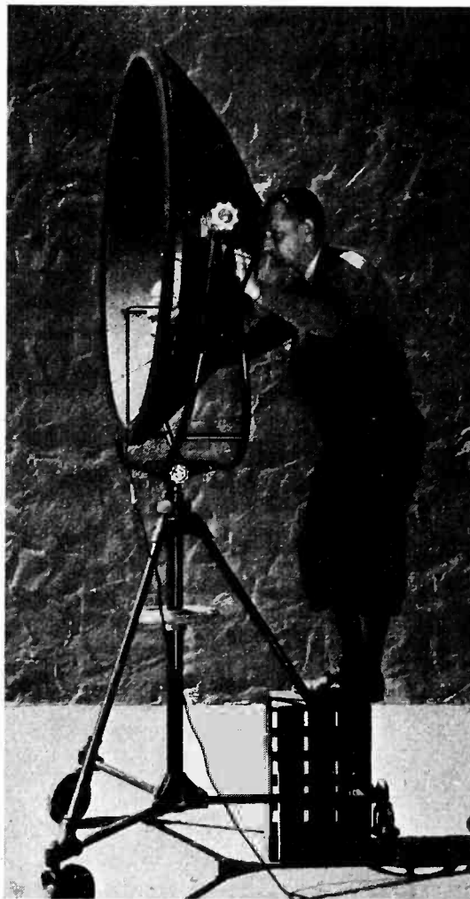
Developed by RKO Studios, Hollywood, this parabolic reflector with microphone placed at the focus is used for long distance pick-up in recording sound pictures
