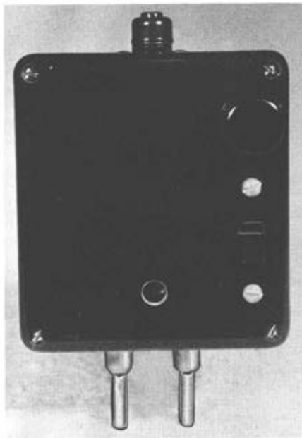
Rear view of the sound level instrument. Note that the miniature volume control potentiometer and the slide-type power switch are attached to the right of the back plate of unit.
