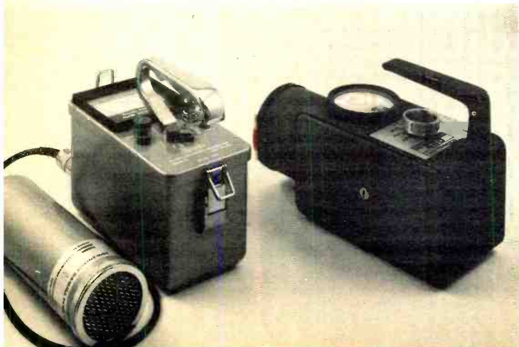
Fig. 1. (Left) Eberline Instrument Corporation's scintillation type and (right) Victoreen Company's ionization chamber are two other survey meters used to detect x-rays from TV sets.
