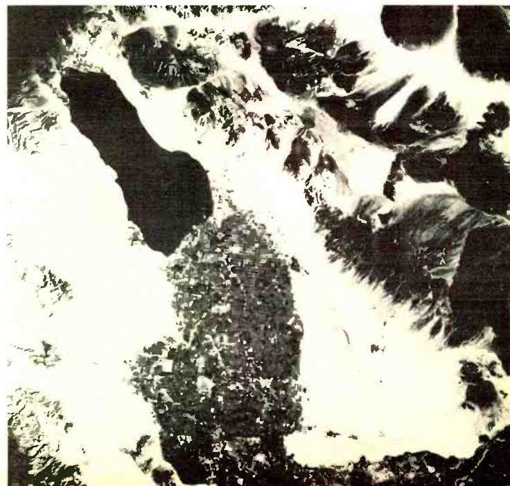
An infrared picture, originally in color, taken from Apollo 9 command module in earth orbit defines cropping patterns in the Imperial Valley of California near the Salton Sea (black body at upper left). ERTS will produce similar data of entire U.S.
