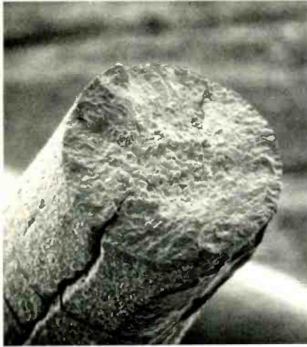
SEM photomicrograph showing stress corrosion fracture in titanium alloy wire (left). Magnification is only 100X; however, photos of opaque objects are not possible with conventional electron microscope. A 2000X enlarged photomicrograph (right) shows the metallurgical structure of end of wire.
