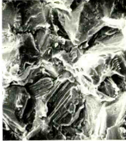
SEM photomicrograph showing stress corrosion fracture in titanium alloy wire (left). Magnification is only 100X; however, photos of opaque objects are not possible with conventional electron microscope. A 2000X enlarged photomicrograph (right) shows the metallurgical structure of end of wire.
