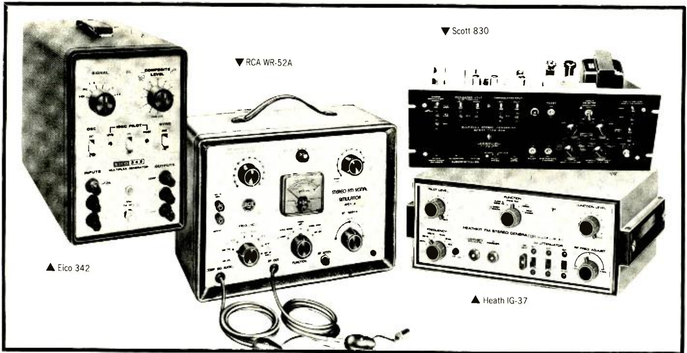
A grouping of stereo-FM signal generators for adjusting FM tuners and receivers.
