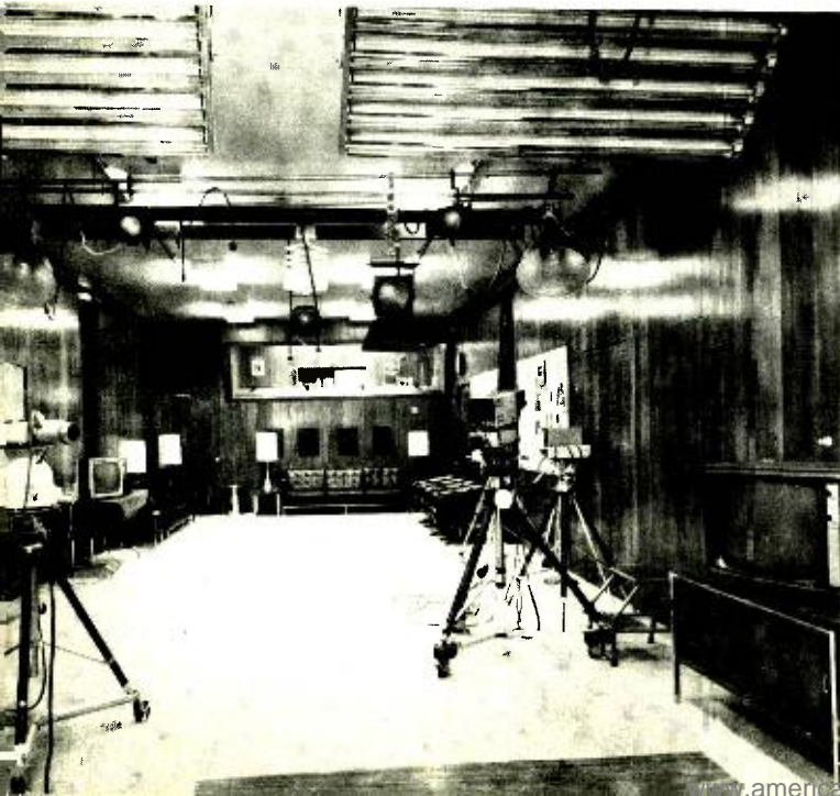
Fig.4. A CCTV studio system set up by Philips Broadcast Equipment Corp. Note the control room in top background.
