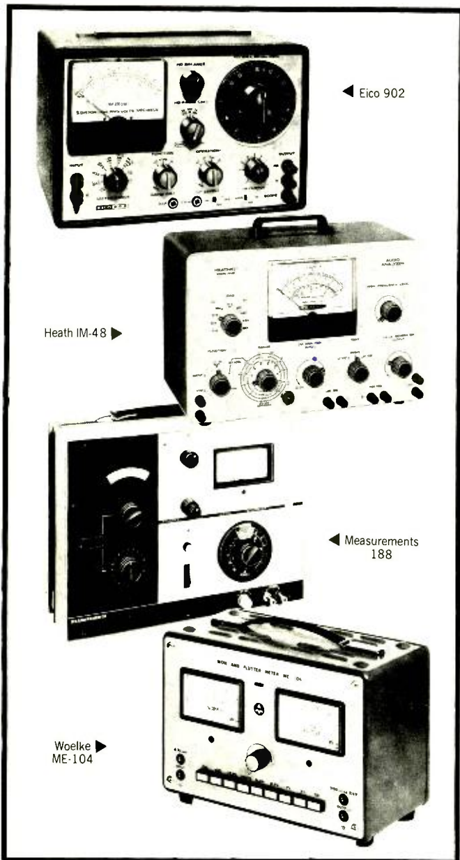
Pair of distortion meters, an FM signal generator, and a wow and flutter meter.
