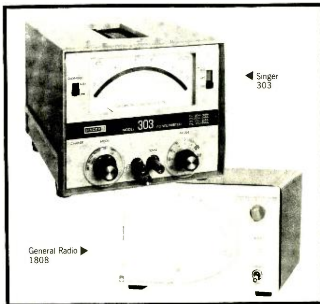
Laboratory-grade high-sensitivity a.c. voltmeters for signal-level measurements.
