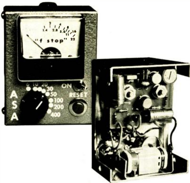
Fig. 1. Front and rear views (with the cover removed) of electronic photoflash meter. Meter is calibrated in "f/stops."
