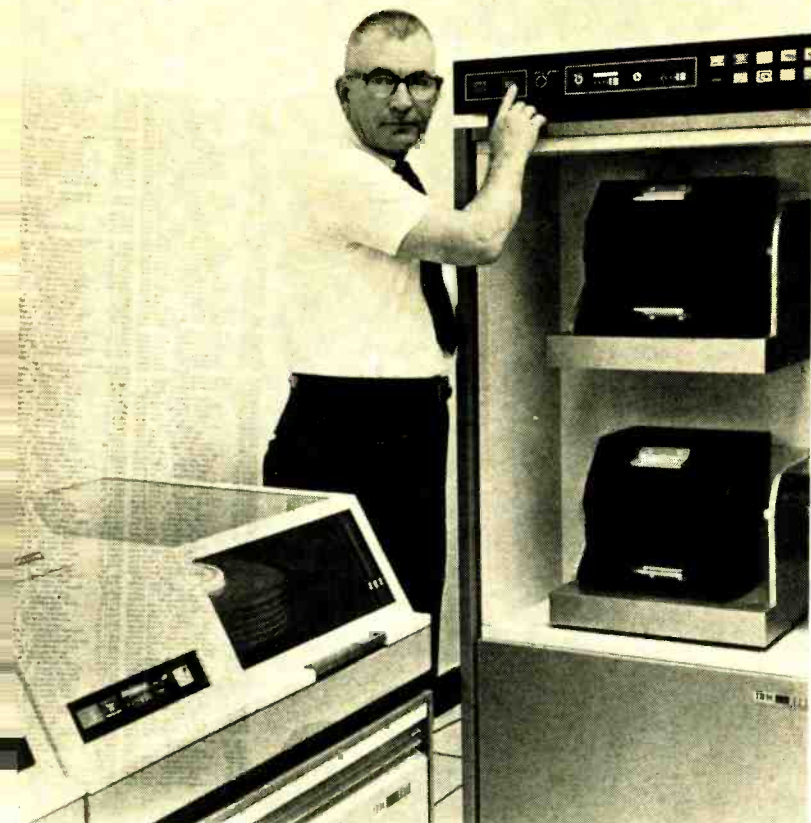
Fig. 1. New electronic photocomposing unit, controlled by an IBM System/360 computer, can set a newspaper page in ten seconds and a full-length novel in approximately ten minutes.
