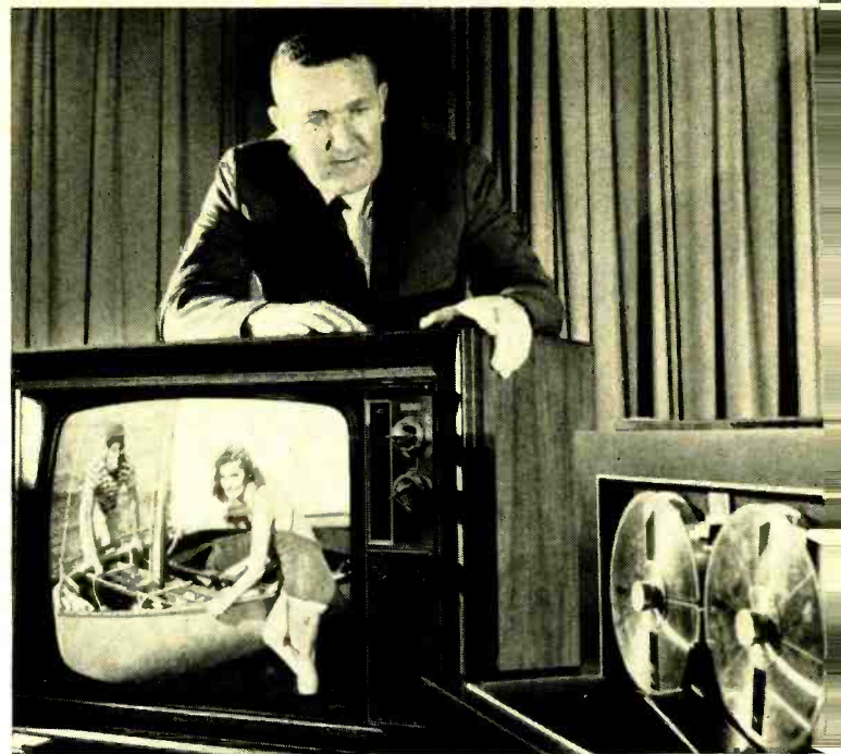
This reel-to-reel tape player, connected to a color-TV set, is the forerunner of a cartridge model scheduled for 1972.
