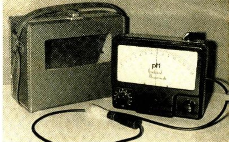
Fig. 1. A portable battery-operated pH meter that is used by electronics technicians who specialize in marine work.
