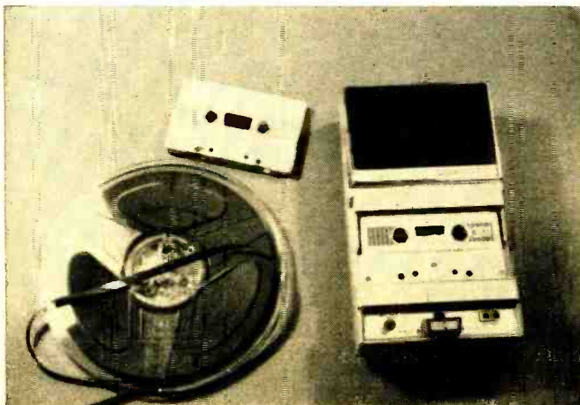
Cassette is compared with an ordinary 7-inch open reel of tape. The portable cassette recorder shown at right is not very much larger than the 7-inch reel of tape.
