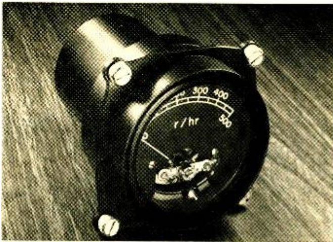
This Eberline & Associates meter is used in systems where it is necessary to continuously monitor high radiation levels.
