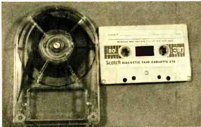
Cassette tape cartridge is compared here with an endless-loop cartridge shown at left. The latter will operate in only one direction and it cannot be operated at high speeds.
