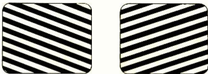
Fig. 5. If the out-of-sync lines slant downhill, as shown at the left, then the horizontal oscillator is running fast. If lines slant uphill, as at right, oscillator is running slow.
