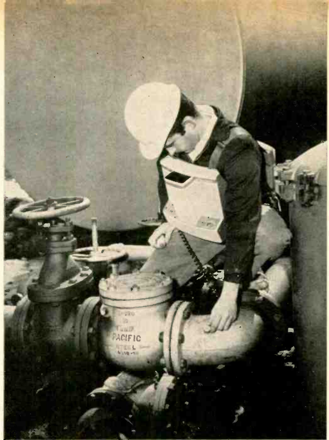
Battery-operated ultrasonic flaw detector and thickness measurement instrument can be used in remote or hazardous areas away from a.c. User's hands are free for climbing or testing.
