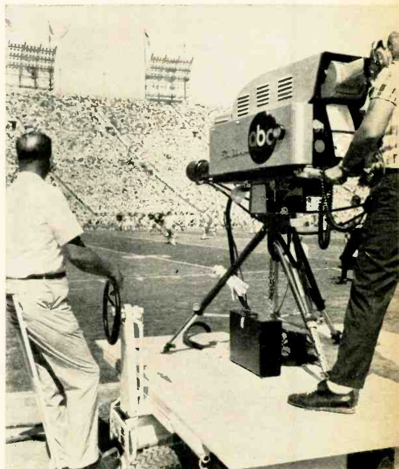
Big color camera provides field-level pictures during last year's UCLA-USC college football game. Camera output feeds an Ampex HS-100 magnetic disc recorder for instant replay viewing and a VR-2000 color videotape unit.
