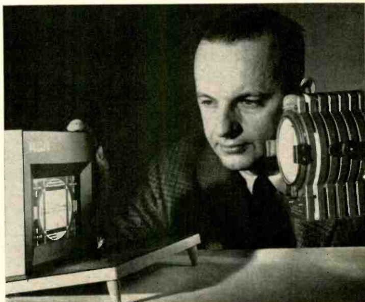
Fig. 3. This high-resolution liquid-crystal test-pattern display gets brighter as the high-intensity light is shone on screen.
