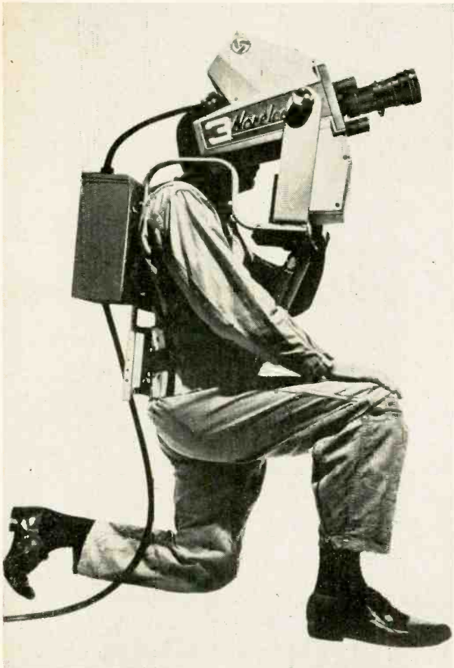
Small mobile color-TV pickup camera uses three Plumbicon tubes whose design utilizes advanced electro-optical principles.
