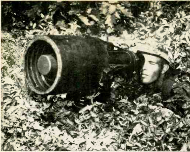
This U.S. Army night-vision sight is used to detect presence of an enemy in faint skyglow or starlight at up to 1200 meters.
