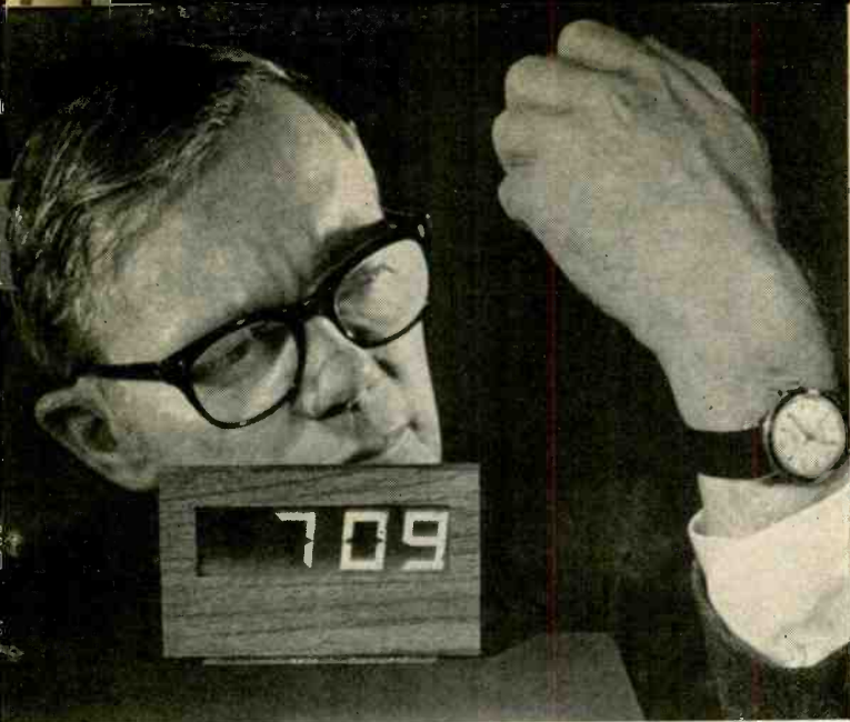
Fig. 1. A liquid-crystal digital clock is shown being checked here against a conventional, "old-fashioned" wrist watch.
