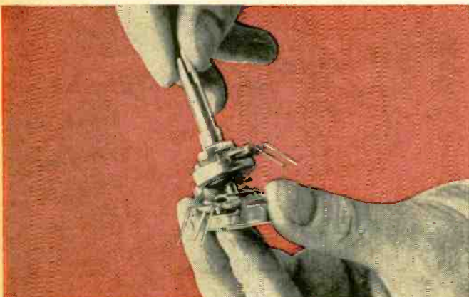
Now push the inner shaft through the front control far enough so you can slide the rear control section in place on the shaft. Finally, attach the rear control section and snap it into place.
