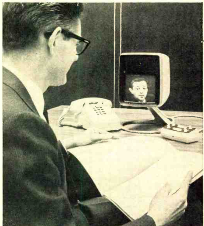
Fig. 4. With the Picturephone set, the user can "zoom" electronically and change the size of field to view a close-up.
