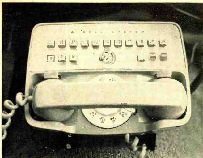
The new MJ mobile system is a full duplex radio. User can dial stations direct from his car on up to eight channels.
