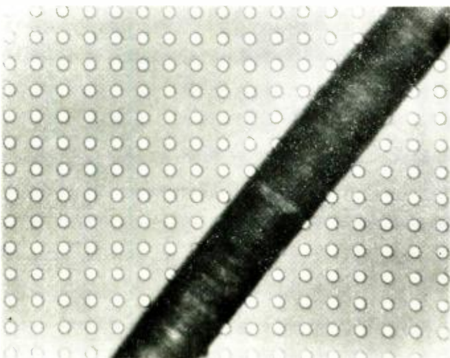
Fig. 1. Section of the photodiode array (white circles) showing their size compared with an ordinary human hair.
