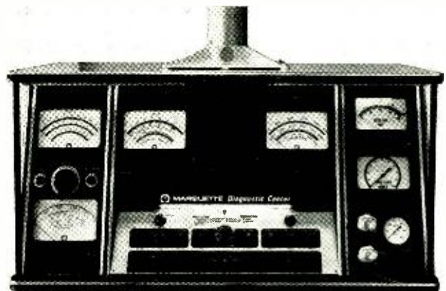
Fig. 6. One type of engine analyzer found in diagnostic centers. This particular one is suspended from ceiling.
