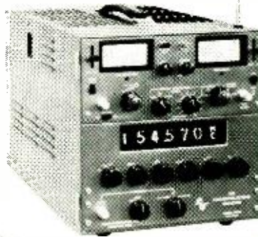
Cushman Model CE-2B FM communications monitor is a direct-reading frequency meter with accuracy better than .0001% over four bands. It also measures FM deviation and generates highly accurate c.w. and FM signals. (Price of the monitor is $3145)
