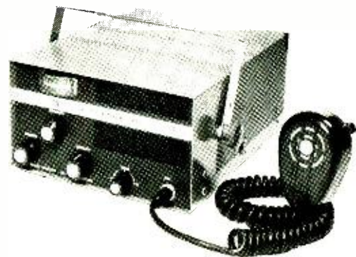
Multi-Elmac "Citi-Fone 55" is a 23-channel transceiver using frequency synthesis and a double-conversion receiver. ($169.50)
