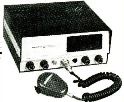
A high v.h.f. band (152-174 MHz) transmitter-receiver. This Aerotron 625U has 25 watts output on two channels, uses FM modulation, and is transistorized except for final. Price $485.
