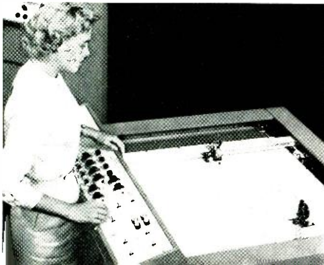
Fig. 9. Digital plotter generating geophysical contour map.
