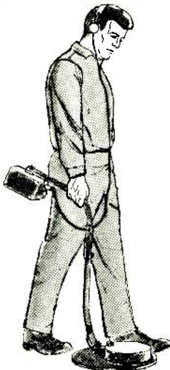
Induction-balance locator uses a more elaborate search loop.
