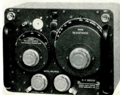
Fig. 12. Radio-frequency bridge for measurements at frequencies up to 60 MHz. At high frequencies, shielding becomes more important, and generator and detector are connected with coaxial cable leads.
