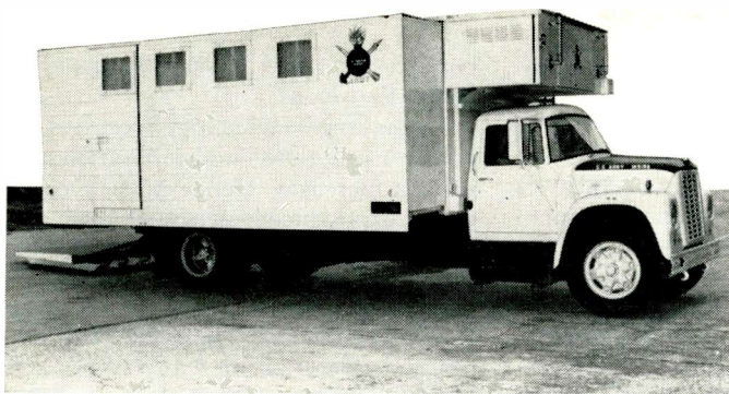
The calibration van can be expanded by opening its sides. Hydraulic lift at rear facilitates moving heavy equipment.
