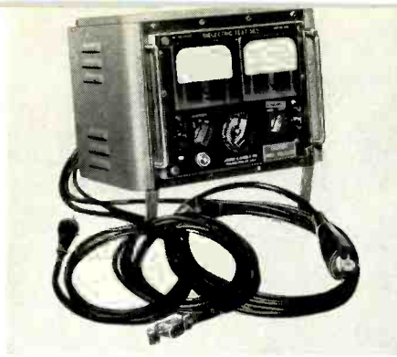
Fig. 6. Biddle 5-kV dielectric test set such as would be used to measure dielectric strength between winding or to case.
