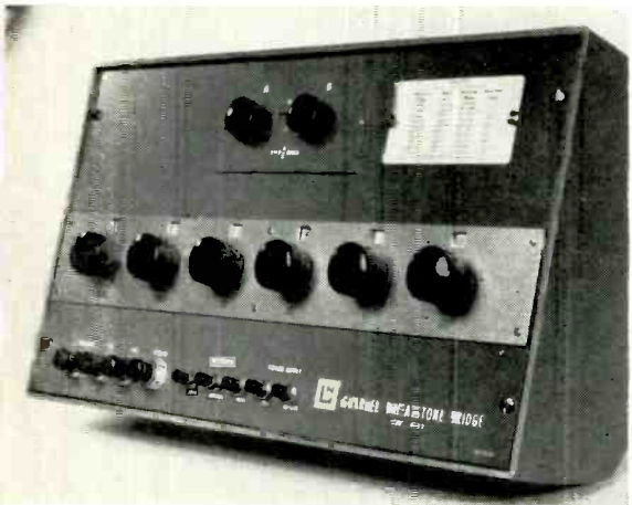
Fig. 9. Leeds & Northrup Wheatstone bridge for highly accurate resistance measurements can check resistors from 1 ohm to over 11,000 meg to 6 significant figures.
