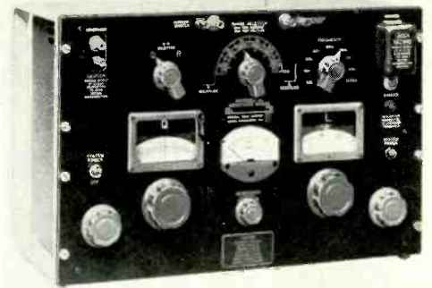
Fig. 7. This incremental-inductance bridge measures the inductance of coils over a wide range of d.c. and a.c. excitation.
