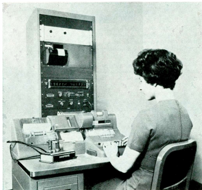
Fig. 4. The automatic capacitance bridge in the middle of the relay rack is the nerve center of this system which measures capacitors and punches values on IBM cards. Operator can punch in supporting data. The bridge is fully automatic. As soon as the operator connects the unknown to bridge terminals (by means of jig on desk at left), the capacitance and loss are indicated, on illuminated readout, with units and decimals.
