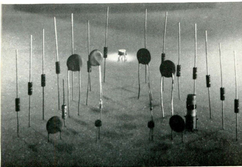
Fig. 1. The linear IC (in spotlight) replaces 26 components shown, besides the many soldering points formerly required.
