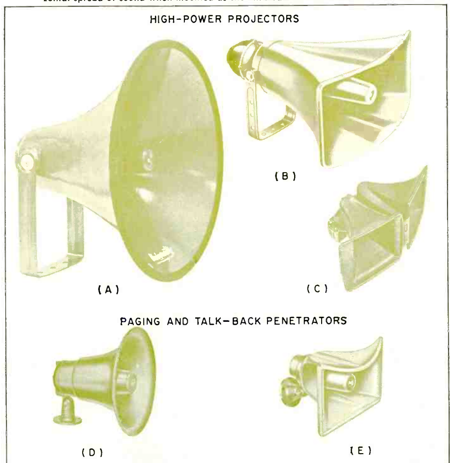
Fig. 3. Standard horns at (A) and (D) produce symmetrical sound patterns. Horns at (B) and (E) have been specially shaped to produce a greater horizontal spread of sound when mounted as shown. Dual horn at (C) has same effect.
