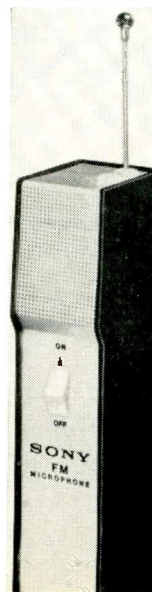
Fig. 2. The Sony CRT-10 is typical of the units operating in the 88-108-MHz FM band.
