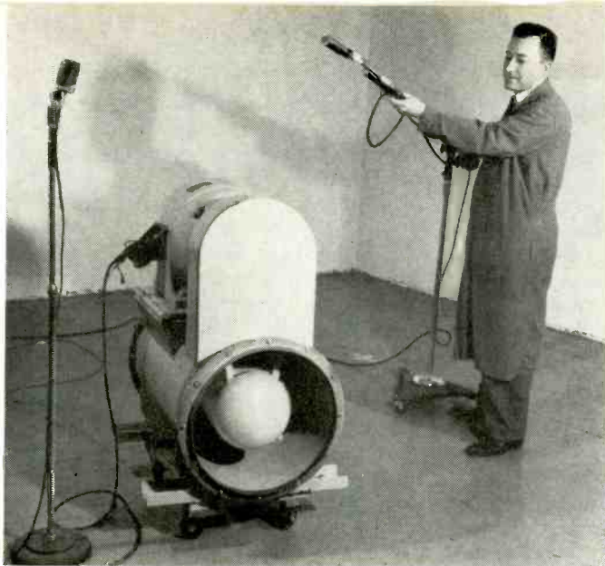
Co-author Wasserman is seen setting up a quality-control test in a reverberant room. Sound-pressure levels produced by an assembly known to be in good condition are being measured. When used in production-line testing, this standard will be used as a comparator against which other similar assemblies will be checked to reject those with faulty bearings, stator or rotor assemblies, or other defects revealed by their sound spectra.
