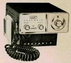
can operate fixed with an optional a.c. power supply.
