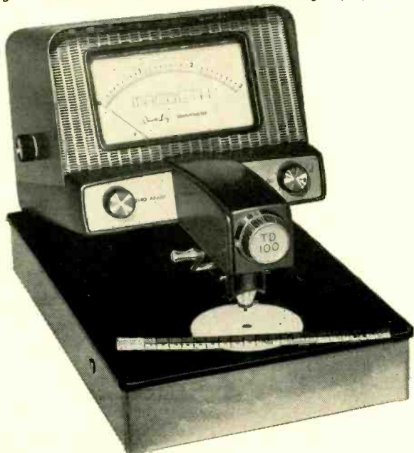
Fig. 3. Transmission densitometer measures image opaqueness.
