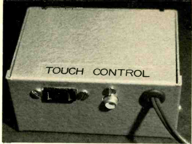
Circuit is built into a 4" x 2" x 2 3/4" metal box. Lamp or low-wattage appliance is plugged into convenience outlet while touch-plate(s) is connected via the phono plug.
