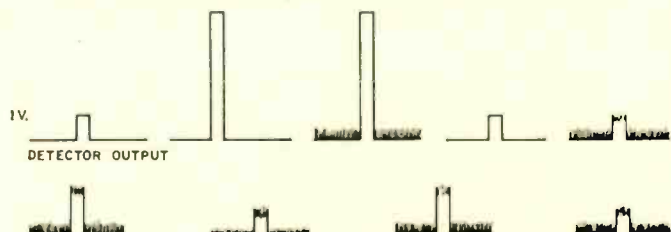
Fig. 5. Detector outputs. Top row, left to right: output, no visible noise; increased gain, still no noise; same condition, noise visible, shows adequate gain; signal reduced to original 1-volt level, noise disappears, signal good; noise level approaching that of signal. Bottom row, left to right: adequate gain and noise figure; gain not improved but noise reduced; same as last case but with additional gain after first stage, over-all signal still good; last condition shows maximum sensitivity (tangential sensitivity) when bottom of noise in pulse is equal to top of noise outside.
