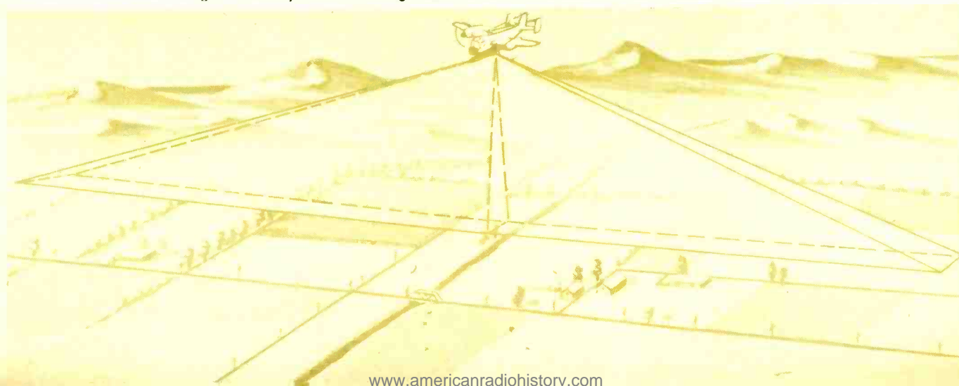
Fig. 2. Geometry of a side-looking radar that has been installed on a reconnaissance aircraft.
