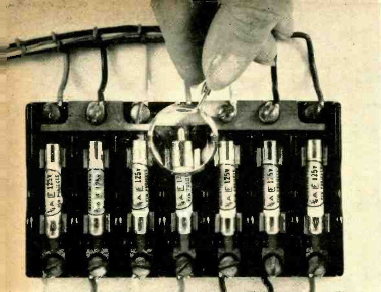
A group of medium-lag indicating fuses is shown. When this fuse blows, the silver-plated indicating pin extends from the end of the fuse. This serves as a visual indicator. The pin can also be used to actuate an audible alarm circuit as well.
