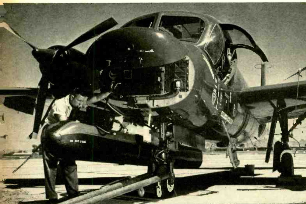
Fig. 1. Side-looking radar installation on an Army Mohawk aircraft. Notice the long cigar-shaped radar antenna housing mounted beneath the fuselage.
