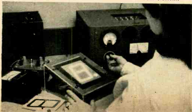
Initial testing of electroluminescent numeric readout element.
