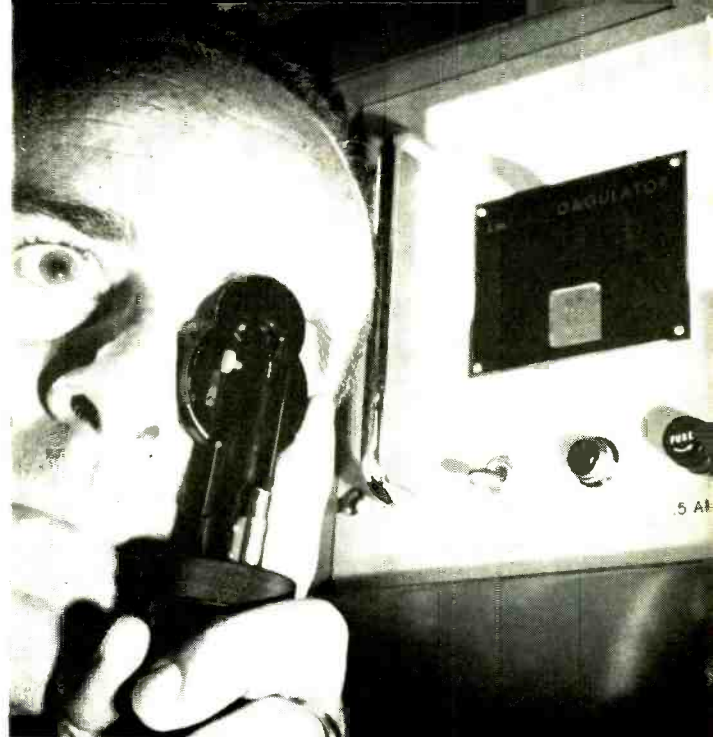
Laser Retina Welder. Light beam from a laser retina welder, developed by Honeywell, is aimed by holding compact ophthalmoscope-like instrument to doctor's eye. Index finger rotates focusing disc correcting for myopic or hyperopic errors. Knurled handle top (above finger) selects proper beam energy. Thumb button fires 500-microsecond burst of laser light into the patient's eye, welding the torn retina by means of the heat scars.
