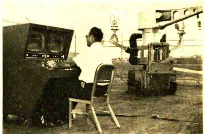
Remotely Controlled Mobile Robot. (Above) The Mobot, manufactured by Hughes Aircraft, is sent through final checkout before delivery to the National Reactor Testing Station, Idaho. Here it will perform clean-up operations. Control commands from operator's console (left) are carried through a cable permitting vehicle to rove up to 500 feet away. TV monitors allow operator to see what robot's closed-circuit TV cameras see . . . Sonar Picture Taker. (Left) Shown entering the water for underwater tests, this Westinghouse sonar search vehicle can map the ocean floor at depths down to 20,000 feet. Information from the vehicle is transmitted by coax to a surface ship, which carries the display equipment and tows the vehicle at speeds up to 4 knots. The "side-looking" sonar has a range of 2400 ft. at right angles to the direction of tow and produces detailed pictures.
