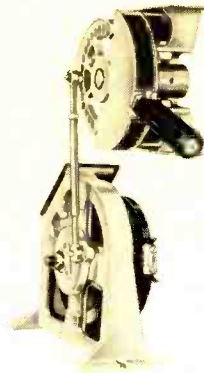
A 2500-watt auto-transformer dimmer designed for manual operation through a drum and lever and a gear drive.
