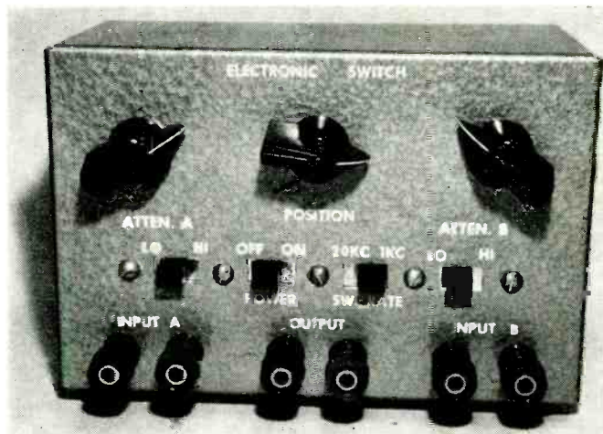
Fig. 3. Author's switch was built in metal cabinet, six inches wide.
