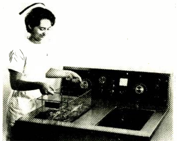
A commercial ultrasonic cleaner with integral generator, transducers, and tank operating with an automatic cleaning and rinsing cycle. This unit is used for cleaning surgical instruments.
