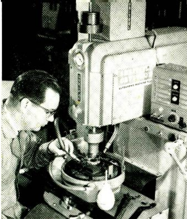
This type of ultrasonic drill (machine tool) is used for a wide variety of applications—drilling, slicing, dicing, and machining.
