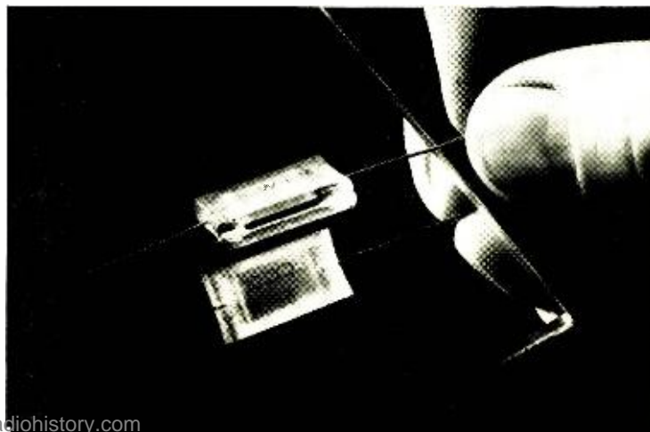
Fig. 1. These monolithic, glass dielectric types produced by Corning can withstand severe environmental conditions.
