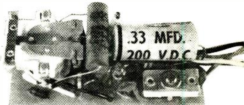
The touch-control circuit is built around a small printed board. The Dynaquad is hidden in this photo. It is located directly below electrolytic capacitor shunting the relay.
