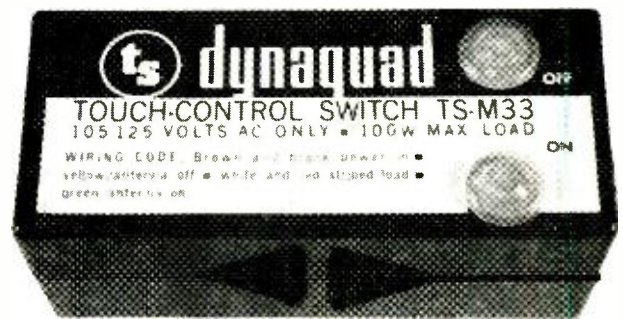
The complete touch-control circuit is contained within plastic box only 3" x 1 1/4" x 1 1/4". The two hole plugs at the right may be removed for readjustment of the trimmers if required. This unit will switch up to 100 watts via a built-in relay.
