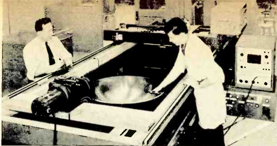
Contract inspection of metal parts by means of ultrasonic tester shown at right.
