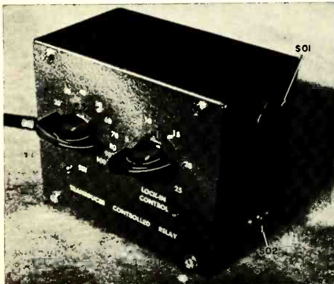
Over-all view of the relay unit built into a 5" x 4" x 3" cabinet.
