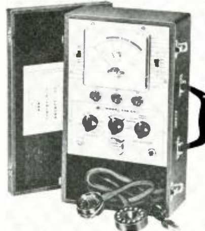
Fig. 2. Model 440, by B&K, is a popular picture-tube tester and rejuvenator.
