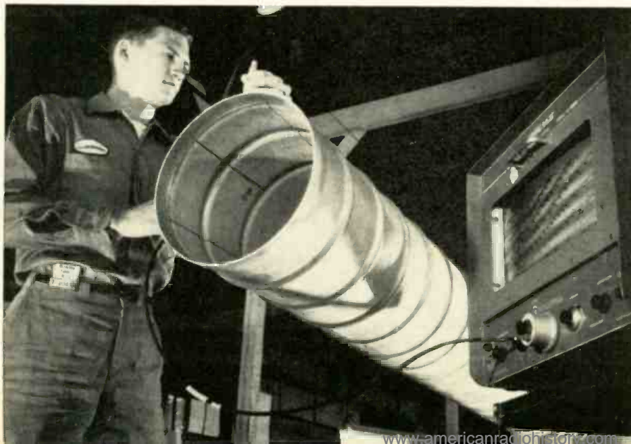
Seamless aluminum tubing used in Titan missile is measured with ultrasonic thickness tester. Instrument requires access from one side, provides .1% accuracy.
