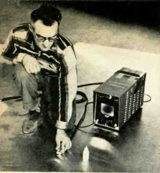
Pulse-echo flaw detector being used to inspect steel plate.
