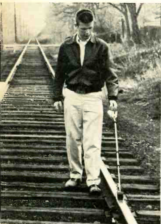
New transistorized ultrasonic rail flaw detector operates on batteries, weighs only 5 pounds. Change in audible tone in operator's headset signals presence of flaw in the rail.
