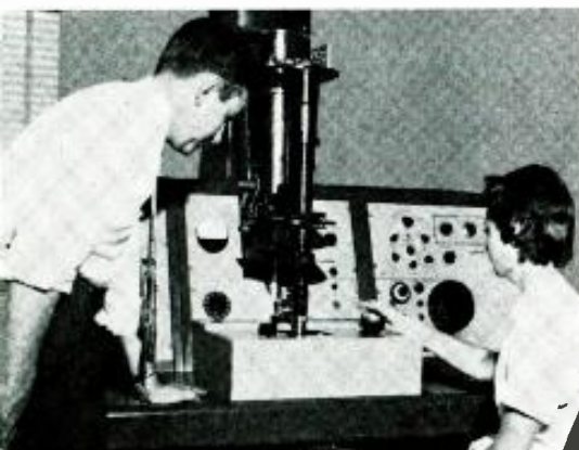
Fig. 10. The "Cytoanalyzer" automatically inspects cervical smears. ▼
