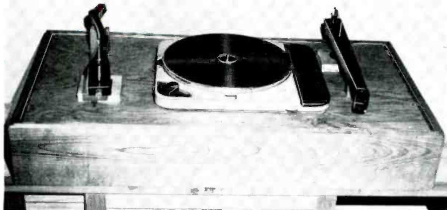
Fig. 1. Over-all view of record-player mounting arrangement described in the article. A pair of home-built tonearms complete the author's playback system.
