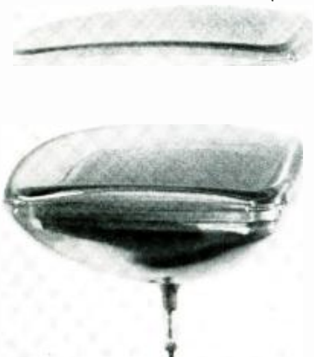
Fig. 1. The glass shield is formed to curve around the faceplate of the tube.
