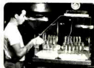
Guns await final assembly in this pressurized plastic housing. Blower at top maintains pressure, prevents dust from entering housing.
