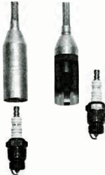
Shields for fitting over spark plugs. Resistor plugs may be used for noise suppression. One of shields has been cut away (at right).
