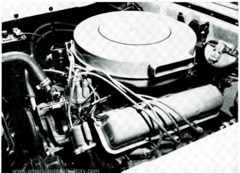
Auto engine equipped with complete filtering and shielding to minimize electrical noise.
