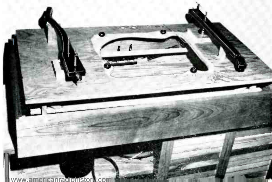
Fig. 2. Top view of the suspension system with the record player removed.
