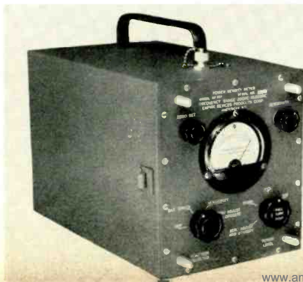
Fig. 1. Typical power-density meter (Empire Devices Products Corp.) with a frequency range of from 200 to 10,000 megacycles.
