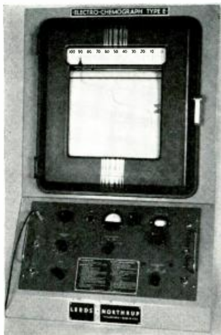
Fig. 2. This automatic polarograph connects to the cell in Fig. 3. The chart has recorded 2 current waves (see text).
