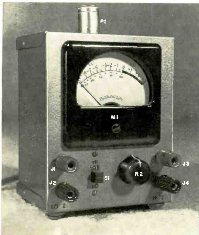
Completed vu meter. The plug-in attenuator pad is at the top of the cabinet. The "Hi-Lo" switch determines which input to utilize.
