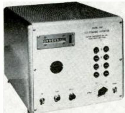
Fig. 5. A totalizing counter containing two decades. Register and lamps show total count.
