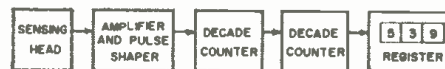
Fig. 4. Decade counters reduce the pulse rate to low value which register can follow.
