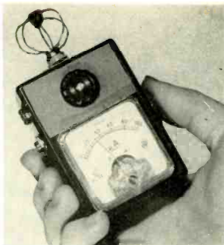
Fig. 6. Model of the Richardson dosimeter built by author. Three small wire loops, each terminated in 10-megohm resistors, act as pickup antennas for the instrument.
