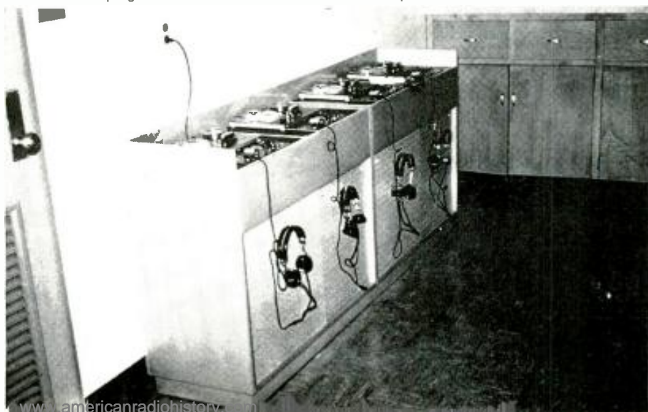
Fig. 4. This corner of the control room shows four of ten tape players that feed master programs to individual booths. A turntable provides an eleventh channel.
