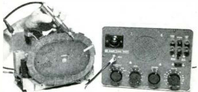
Fig. 2. Detector probe near antenna yields audible signals.
