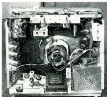
Fig. 3. This Hoffman chassis comprises 4 accessible assemblies framing the CRT.
