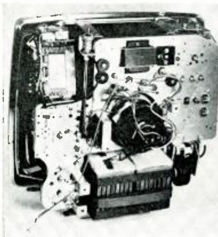
Fig. 4. Transistors and other parts are all on rear deck of Motorola's "Astronaut."
