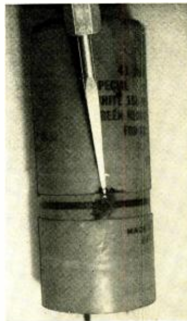
Fig. 6. The pointer indicates stain on capacitor case from electrolyte leakage.
