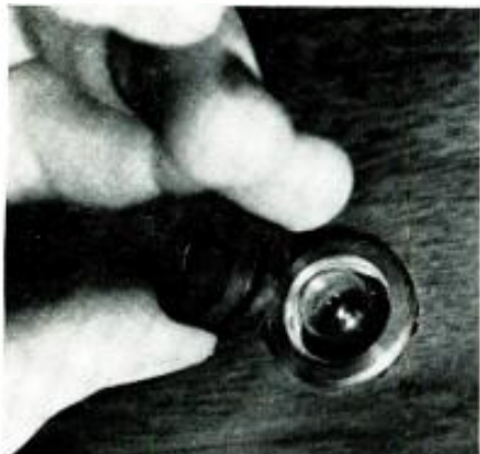
(Above) Using grommets as "bumpers" to protect pilot lights. (Below) In emergencies, grommets make good pilot-light pullers.
