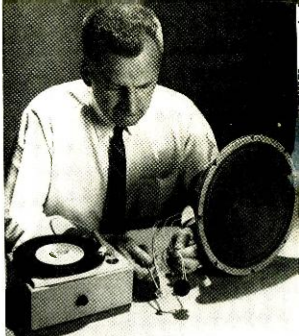
Molecular electronic phono system. Preamp is tiny unit in engineer's right hand, and 5-watt 0-20,000 cps power amplifier to drive speaker is in small black box in left hand.
