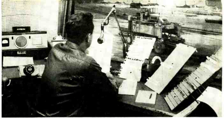
Fig. 2. The central material-handling dispatcher, located at the Gambrinus plant, directs the movements for a large fleet of vehicles. He is shown routing a straddle carrier, which is visible through the window of his booth.
