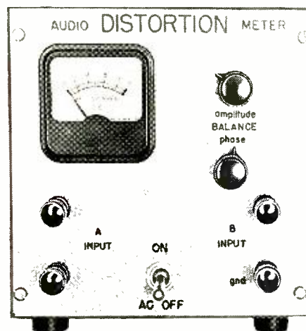
Front-panel layout that is employed in the author's distortion meter.
